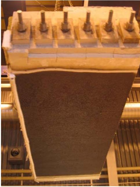
Photograph: One of the 3.6m x 1.2m pre-stressed concrete slabs fire protected with 36mm of FireBarrier 135 being after the 2 hour fire test showing the surface to be intact with no spalling having occurred.
